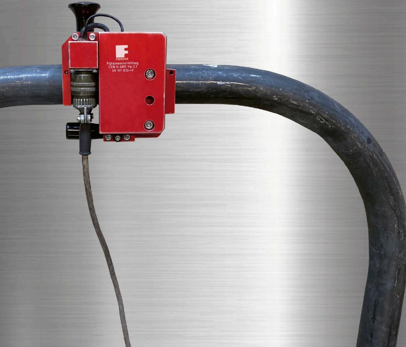
Wrought outlet pigtails are critical components that need rigorous inspection due to their location and intended function. For the identification and determination of creep, we have developed a unique device for measuring pigtails diametrically from the tube outlet to the manifold.
