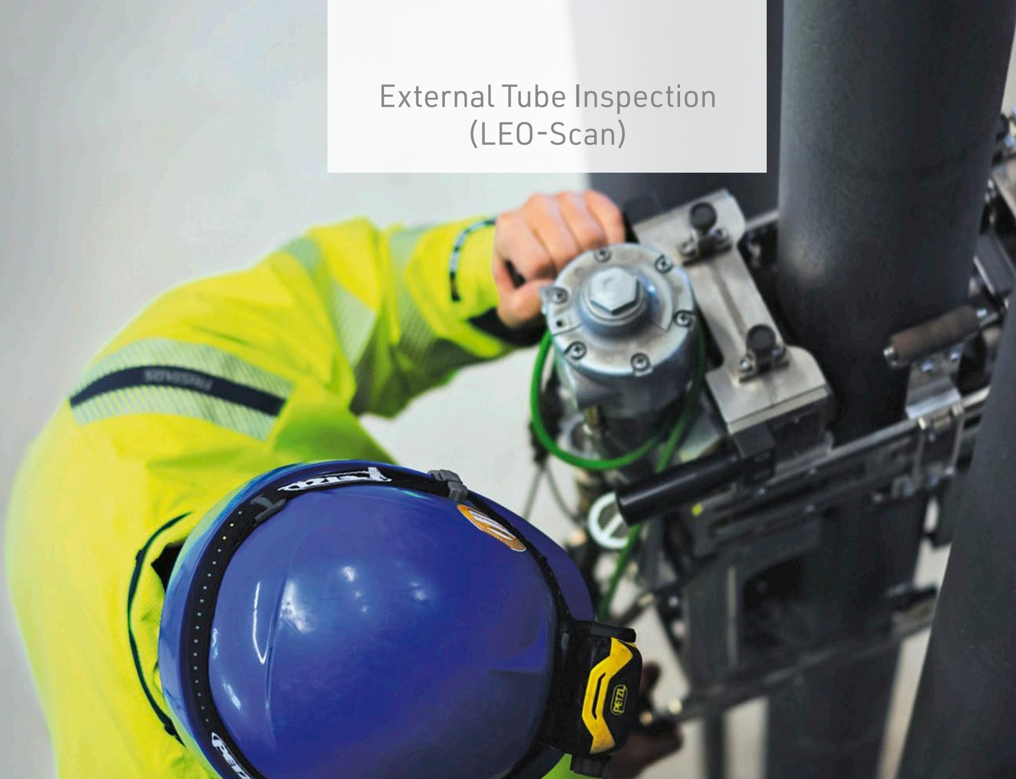
For the purpose of inspecting centrifugally cast reformer catalyst tubes used in steam methane reformers, FOERSTER has developed and built the proprietary "LEO-Scan" system, an inspection carried out from the outside of the tubes, using the Eddy current and Laser technique.
