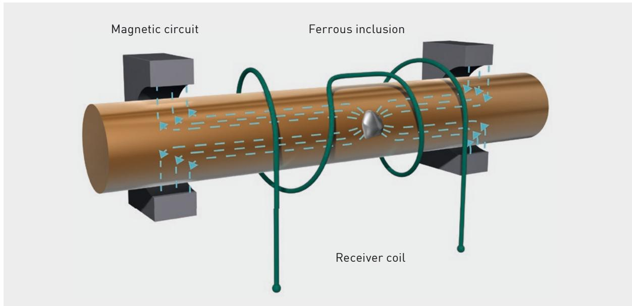
*Principle for the detection of ferrous inclusions*
